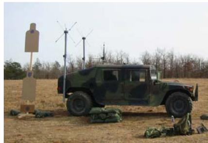
Figure 2: HMMVV with two Boomerang sensors mounted on back
